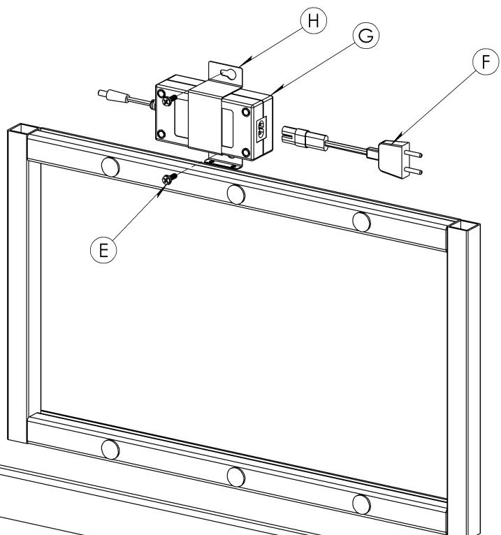
The person mounting the power supply bracket must choose screws etc. that suit the condition of the wall!
