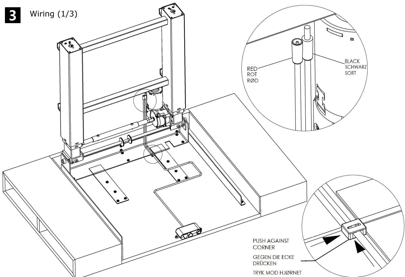
Make sure the wires are not in the way of folding movement - Test the wiring by folding desk down and up before adding wire nails. See page 9 step 1 for folding instructions.
