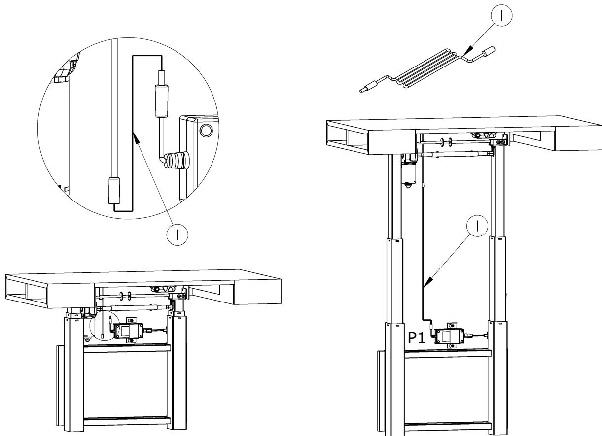
Use the extender wire (I) to connect the red wire and power supply. When the two are connected elevate the desk to maximum height. Then fold the excess wire at position P1. Secure the fold with a cable tie(K).
