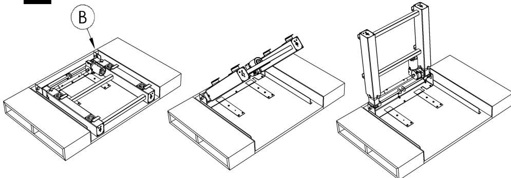
**Fold desk up (a)** Just fold the frame up by hand and it will automatically stay up once it is perpendicular to the tabletop. Once the automatic trigger is activated there will be a click sound.
