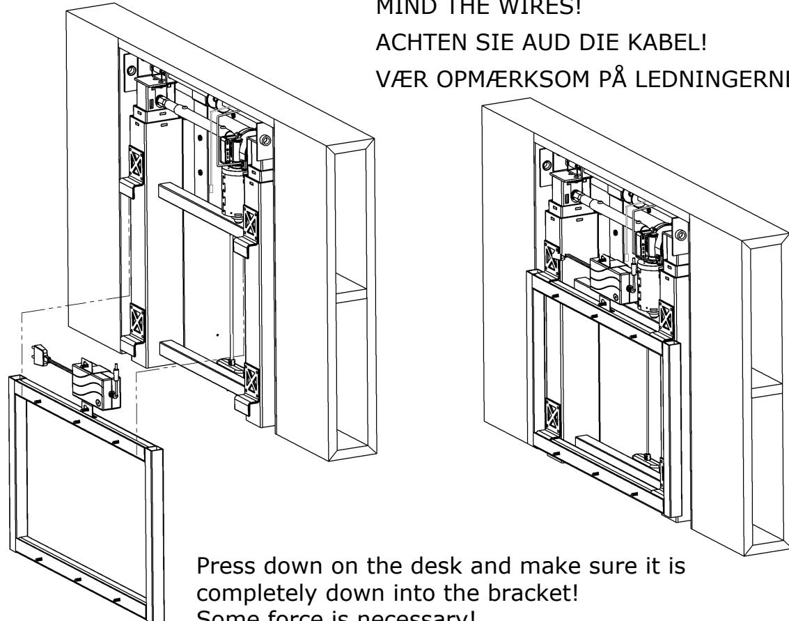
Press down on the desk and make sure it is completely down into the bracket!
