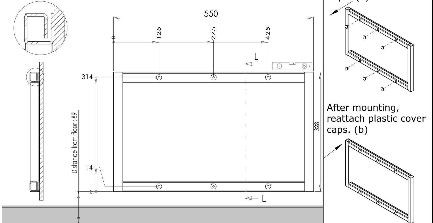
The bracket must be level. **The minimum distance from the floor is 35 mm.**
